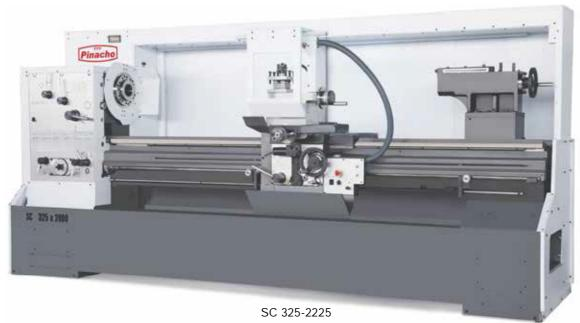
Pinacho lathes type SC is a new series of conventional lathes which comes in sizes from 200-325mm in centre height, and from 750 - 3150mm between the centers. Motor sizes are available from 4-7,5kW. All the machines are standard with variable adjustment of spindle and with 3 gears. The combination of constant cutting speed with electronic variable speed, give these machines a better performance and a much finer surface on the workpieces.
